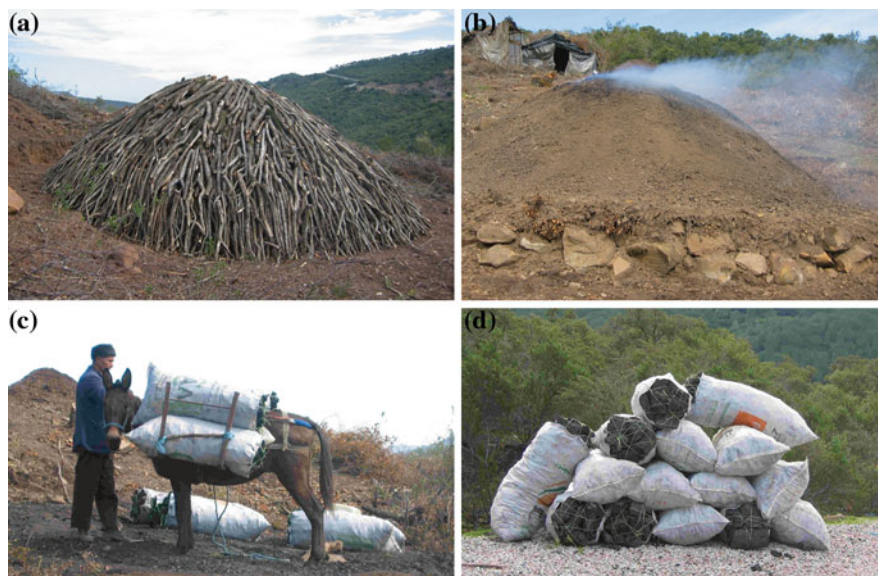
Fig. 9.6 a, b The traditional method of charcoal preparation consists of covering a woodpile with soil and straw, allowing only a small amount of air to enter. The wood sticks burn very slowly in a “cold fire” and become charcoal. c, d Charcoal loaded in bags for transport and sale (Photographs by P. Ovando)
